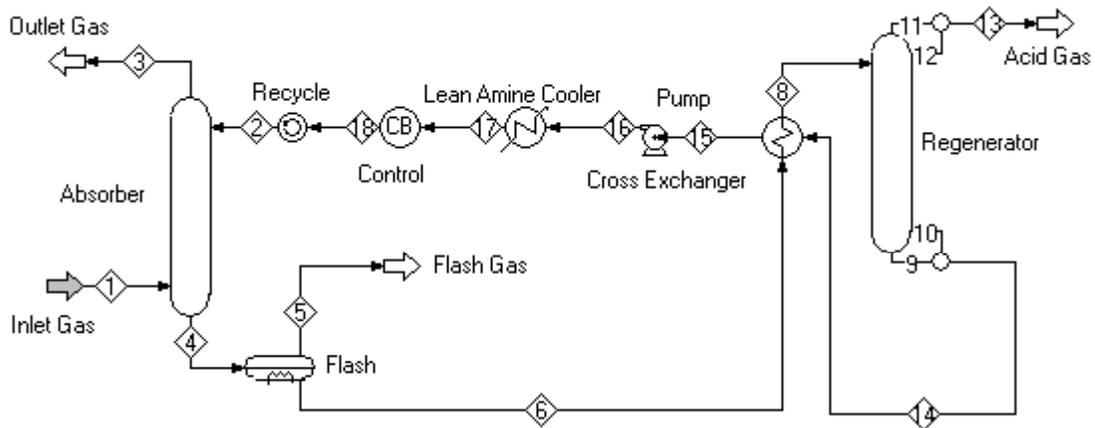
Predicting plant future performance and identifying process limitations are critical in natural gas applications where flows and compositions are likely to change drastically as new wells are brought into production and treating requirements change. This is a case study of an offshore application demonstrating how simulations were used to design an amine plant to accommodate expected (and somewhat unexpected) deviations from the original process conditions (Table 1).
