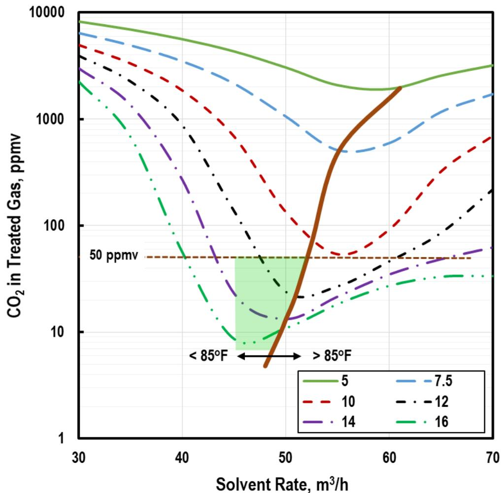
**Figure 1 Treating Response using 50 wt% Total Amine**
