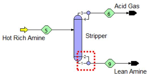
Figure 1. PFD for Kettle Type Reboiler in ProTreat®
