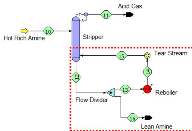
Figure 2. PFD for Thermosyphon Type Reboiler in ProTreat®
