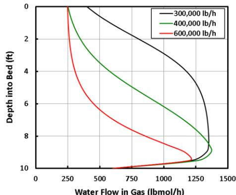
**Figure 5 Water Flow Rates in the Gas**
