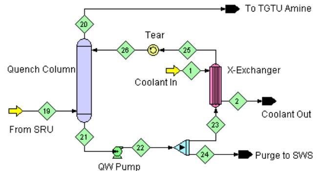
Figure 1 TGTU Quench Column with Quench Water Cooler
