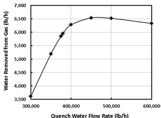
**Figure 3 Effect of Quench Water Rate on Water Removal from Gas**
