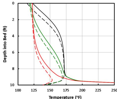
**Figure 4 Temperatures in Quench Tower At 300,000; 400,000, 600,000 lb/h Gas: ———, Liquid: - - - - -**
