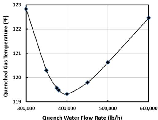
**Figure 2 Effect of Quench Water Rate on Quenched Gas Temperature**
